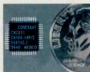
Conextant's new smaller-than-a-dime silicon tuner is aimed at the cable modem market.
