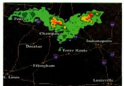
Advanced Designs Corp.'s Dual Doppler feature incorporates radar weather data from two stations in one real-time map.
